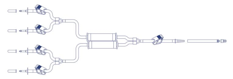
Non-Vented Perforator x4, Click Clamp x5, Hand Pump x2, Stepped Connector with Silicone Tubing Adaptor, Male Luer Lock with Rotating Collar, 270 cm, Internal Diameter: 2 mm, Shelflife: 3 years, 25/Box
